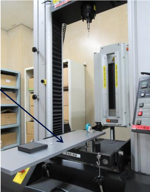
Specimen: Compression molded sheet (0.5mmt)
