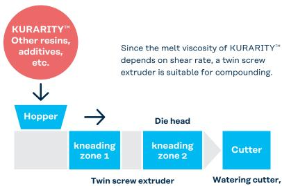
Watering cutter, under water cutter, strand cutter, etc.
