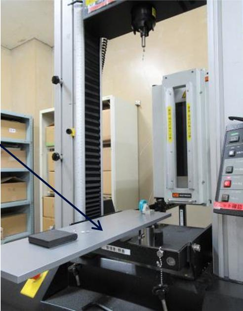
Specimen: Compression molded sheet (0.5 mmt)
