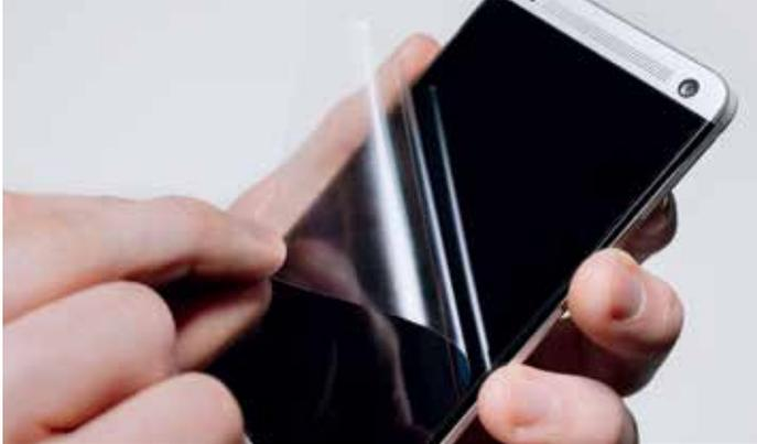
Kuraray has developed material technology that is applicable for surface protection films. The core chemistry is based on styrenic-block copolymers and is known under the tradenames of SEPTON™ & HYBRAR™. When using these products in protective films, they allow design flexibility in customizing tack adhesion, strengthening ultimate tack, and residue-free removal.
