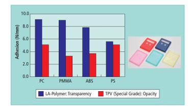
Fig. 8: Adhesion to polar plastics in peel test; photograph shows double moulded samples.
