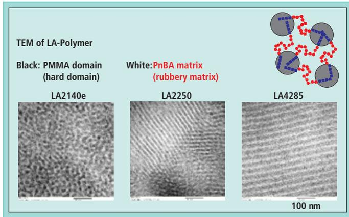
Fig. 3: Morphology investigation of LA-Polymer by TEM (Transmission Electron Microscopy)
