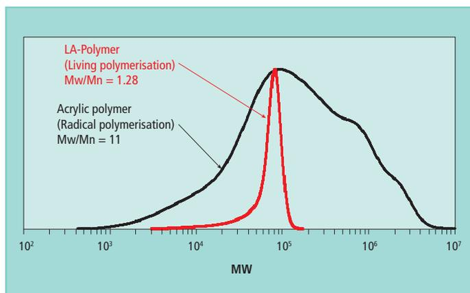
Fig. 2a: SEC (Size Exclusion Chromatography) and molecular weight distribution curves of LA-Polymer and conventionally made PMMA
