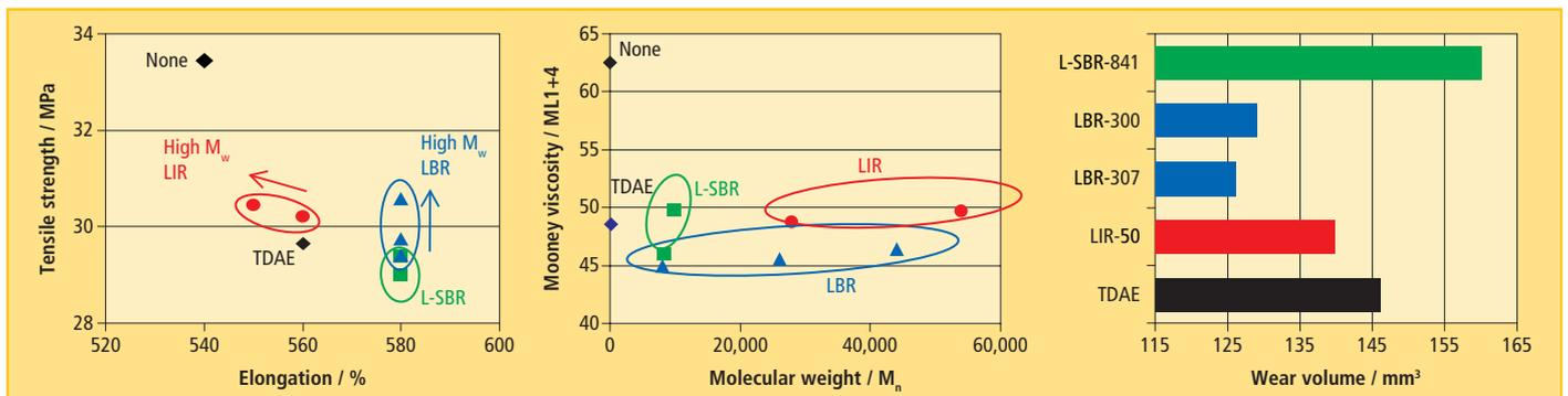
Fig. 4: Viscoelastic characteristics
