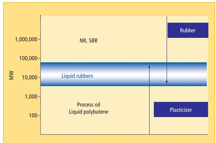
Fig. 1: Molecular weight of liquid rubber
