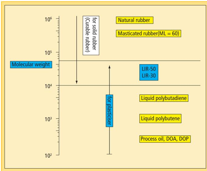
Fig. 1: Molecular weight of Kuraray liquid rubber
