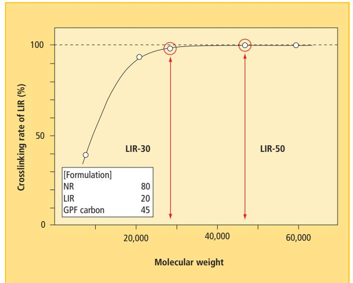
Fig. 2: Molecular weight dependency of crosslinking rate of polyisoprene
