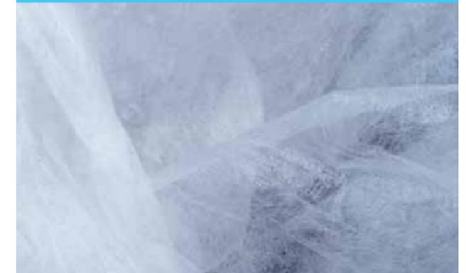
Soft and elastic with low hysteresis and permanent set. Melt blown processable for nonwovens and excellent extrudability for elastic film.
